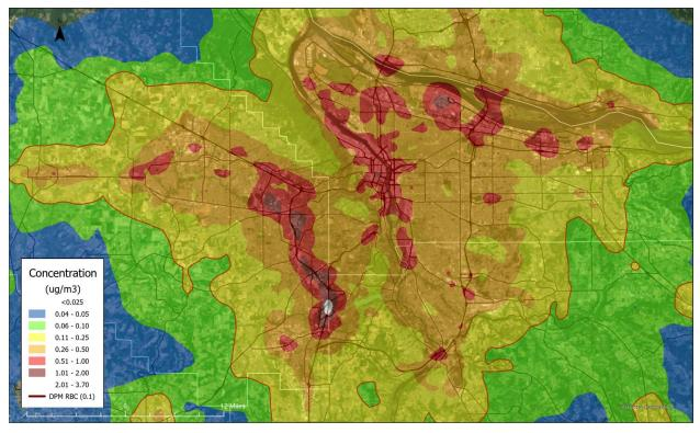
Figure 1. PSU-2020 model of all sources of diesel particulate matter based on Rogers, 2022 modified with up-to-date TriMet bus data provided by TriMet (Table 1).
