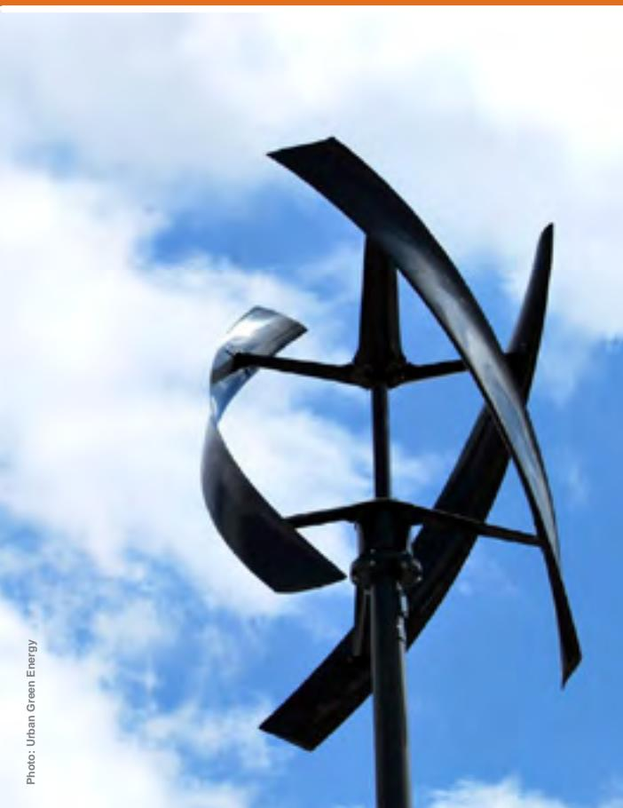
*Vertical-axis wind turbines (VAWTs) offer several advantages over traditional, horizontal-axis wind turbines (HAWTs). VAWTs are highly efficient and do not require as much wind to generate power, allowing them to be closer to the ground where wind speed is lower and where they can be maintained in safer and more efficient ways. They are also omni-directional, meaning they do not have to point into the wind, eliminating the need for wind-sensing and orientation equipment.*
